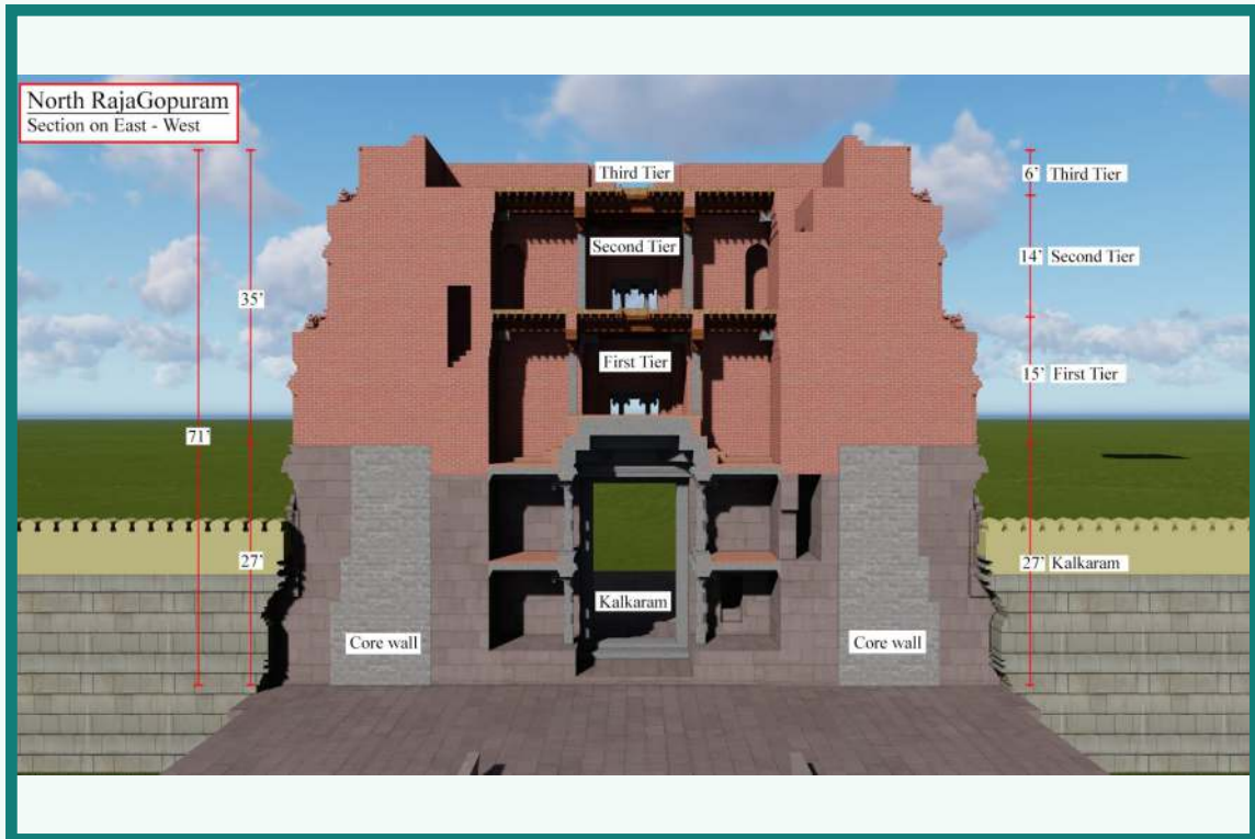
The computer generated 3D model in the existing Mottai RajaGopuram. The inside construction details are also shown.
